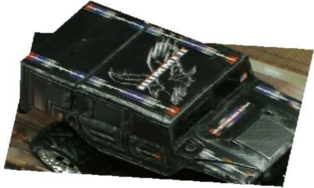
Figure 3. This figure illustrates a texture mapped 3D model of the car obtained by interpolating from the sparse structure estimates generated by FBSfM. Manually assisted feature point matches were also used to generate this result, to ensure display a full 3D model
